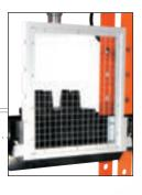
HD cable winch for raising and lowering press bed (50 and 75 Ton only)
