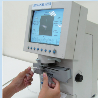
LENS ANALYZER Advanced testing of refractive, astigmatism and optical quality.
