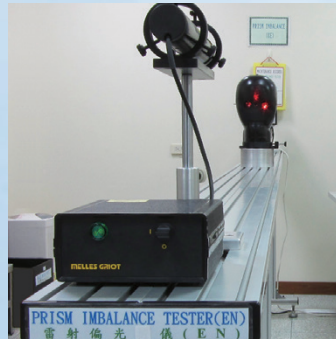
PRISM IMBALANCE TEST Inspects prism power and imbalance of the lenses.
