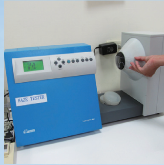
HAZE TESTER Measures the haze (light scattering) and light transmitting properties of the lenses.
