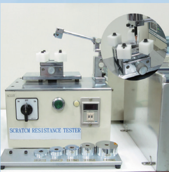
SCRATCH RESISTANCE Measures the scratch resistance of the lenses.
