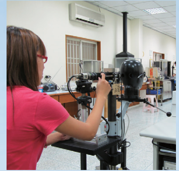
DEFINITION TEST Checks the optical quality, definition, refractive power, and astigmatism power test.
