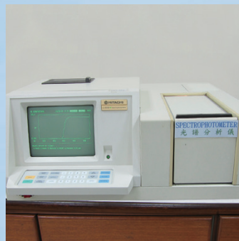
SPECTROPHOTOMETER Examines the ultraviolet radiation and wavelengths of coatings.
