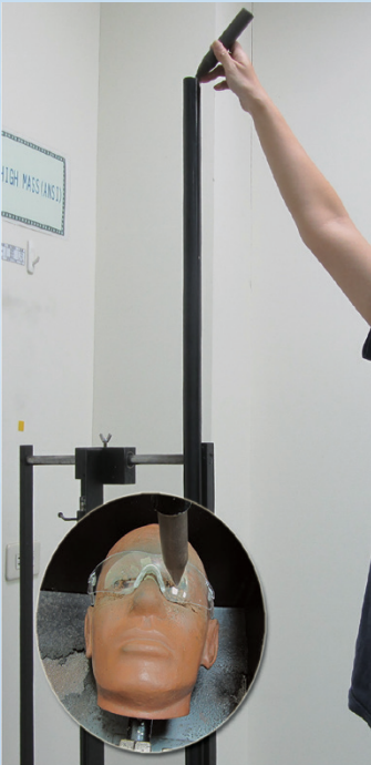
HIGH MASS IMPACT TEST Measures for the level of protection against relatively heavy objects traveling at various speeds.
