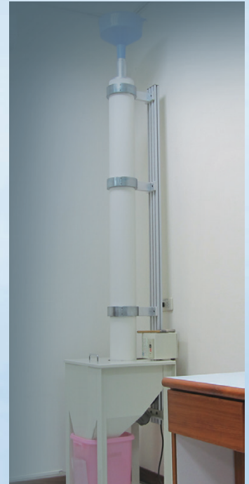
FALLING SAND TEST Measures level of resistance to surface damage by fine particles.
