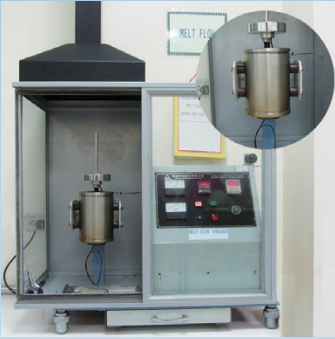
MELT FLOW INDEXER Tests the quality of raw materials.
