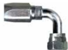
90° ELBOW (LONG STYLE) S.A.E. 37° Female Flare (Swivel)
