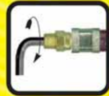
Hold Shell and Tighten Stem With Key
