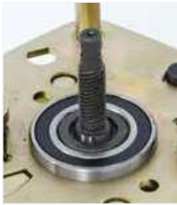
Maintenance free sealed bearings reduce operator effort
