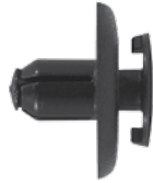
247-111 Std. Pkg. 25 pcs. Head Dia. 20mm, Stem Length: 8mm LEXUS 2000-on Rocket Panel & Garnish Moulding Retainer Fits into 7mm Hole #90467-07168
