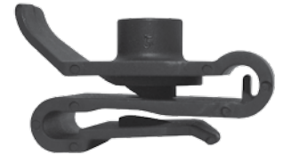
247-844 Std. Pkg. 15 pcs. Screw Size: No.12 (M5.5) LEXUS Black Nylon Bumper & Fender Apron Nylon "U" Nut Width: 20mm, Length: 36mm Center Of Hole to Edge: 14mm Panel Range: Up To 1mm #90467-05114
