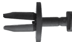
247-411 Std. Pkg. 25 pcs. Head Dia. 21/32", Stem Length: 9/16" GM 1981-on Radiator Overflow Windshield Washer Bottle Retainer Fits into 5/16" Hole #14019226, 14071289 CL Part No: 910-0810, Pieces: 3
