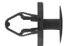
247-423 Std. Pkg. 25 pcs. Head Dia. 19mm, Stem Length: 14mm BUICK Enclave & LaCrosse, Cadillac, CTS, SRX & STS Chevrolet Cobalt, Equinox & Malibu, GM Trucks & Pontiac G5, G6 & Torrent 2003-on Fender Apron Retainer Panel Ran: 2.7mm-5.3mm, Fits into 8.5mm Hole #11609417 CL Part No: 910-0610, Pieces: 4
