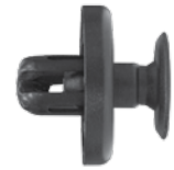
247-503 Std. Pkg. 15 pcs. Head Dia. 18mm, Stem Length: 7.5mm LEXUS 1999-on Front Fender Liner Retainer Fits into 7mm Hole #90467-10183
