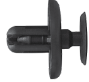
247-228 Std. Pkg. 15 pcs. Head Dia. 20mm, Stem Length: 10mm LEXUS ES300/330 Engine Under Cover Push-Type Retainer Fits into 7mm Hole # 90467-07201
