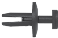
247-464 Std. Pkg. 25 pcs. Head Dia. 5/8", Stem Length: 17/32" FORD Taurus, Topaz & Sable 1989-on Black Nylon Push-Type Retainer Fits into 1/4" Hole #N805231S CL Part No: 910-0790, Pieces: 4
