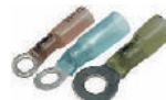
Heat Shrink Insulated Translucent, adhesive-lined polyolefin tubing allows visual inspection, prevents wire corrosion and provides a waterproof seal. Conforms to automotive manufacturers' specifications for wiring repairs, necessary for maintaining electrical warranties.
