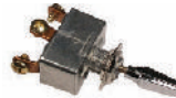
Momentary SPDT Toggle Switch Controls two single wire circuits, permitting only one circuit to be energized at a time. HD Die Cast. 6-12V 50A 1/2" Mount Hole On-Off-On
