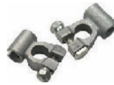
Split Barrel Each battery terminal comes with a nut and bolt giving tight connections to battery post for solid electrical contact. Material: Brass Wire Application: Solder 2/0 - 3/0 AWG
