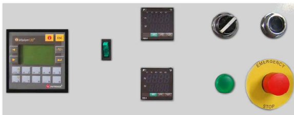
Unit Controls with Emergency Stop
